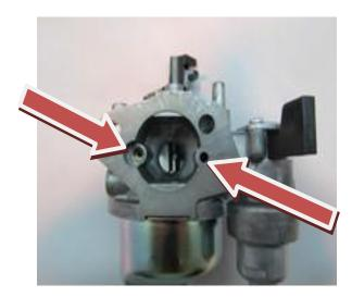
**F.** Main nozzle will be checked with a No/Go Gauge (0.424") If gauge goes over dump tube carb is illegal. This is best measured using a 0.452" rod type gauge with a 0.424" flat area to be used as a go gauge.
