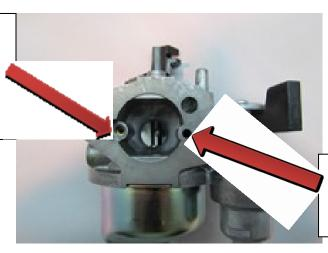
The hole at the end of the arrow is the Main Air Jet hole and will be checked using a pin type no-go gauge.
