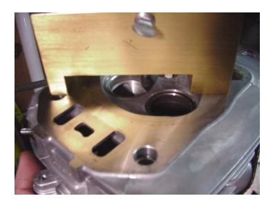
D. Thickness of head. This will be measured from valve cover surface to head gasket surface at the side at a position in line with upper intake & exhaust flange bolt.
