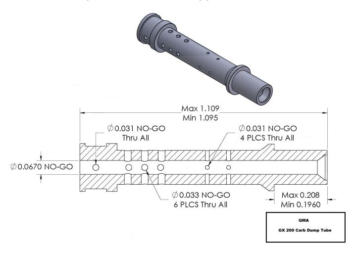
Must be stock Honda GX200 Dump Tube. NO ALTERATIONS
