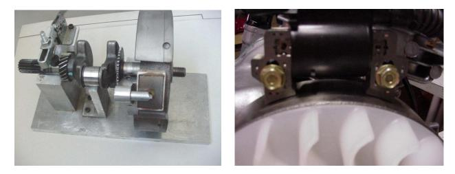
F. All nylon blades on the cooling fan must be intact. If missing fins due to normal breakage and hasn't been modified, Take out of service.
