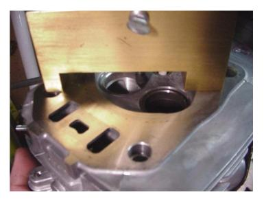
C. Measure from surface of head to lowest machined area in the bowl of the port. This dimension will be: Intake: 1.130" Min to 1.150" Max depth
